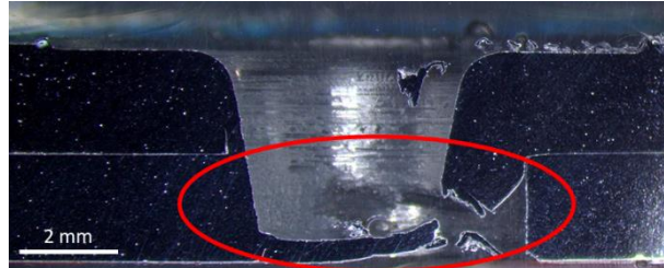
Figure 14. Macrosections of incomplete back-filled specimens with pilot holes at magnesium plate only
