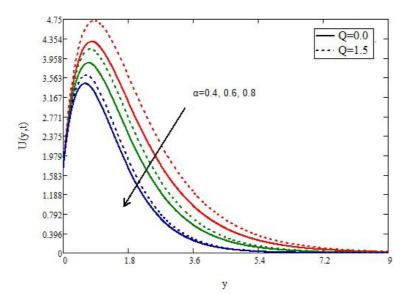
**Figure 2.** Effect of Q on velocity profile with different values of  $\alpha$ .
