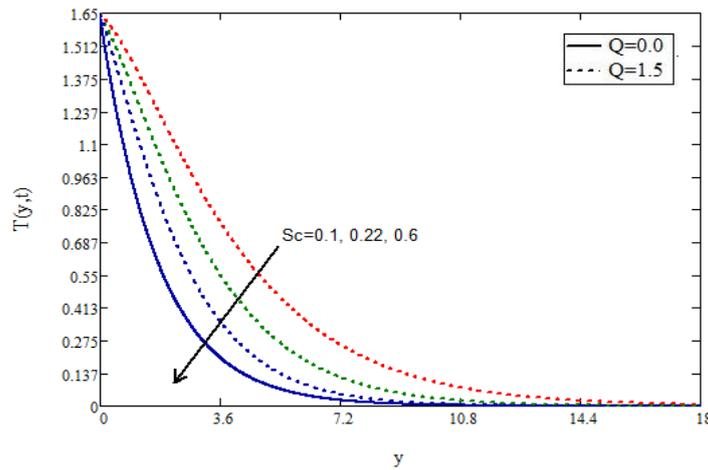
Figure 7. Effect of  $Q$  on temperature profile with different values of  $Sc$
