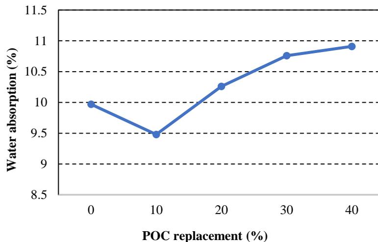
Figure 5. Water absorption in mortar with varying percentages of POC
