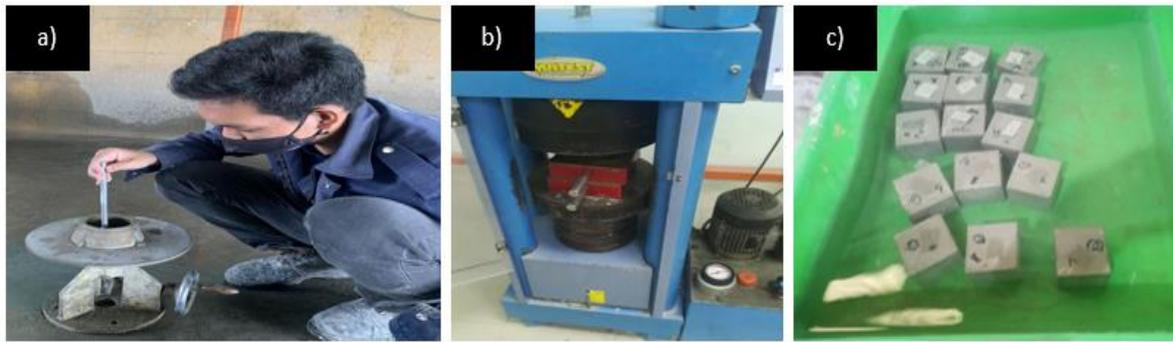
Figure 2. List of experiments a) Flowability test b) Compressive strength test c) Water absorption test
