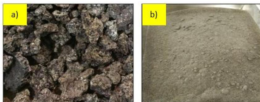
Figure 1. a) POC before crushed b) POC ready to use
