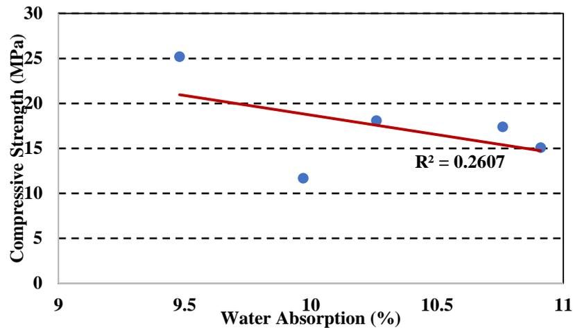
Figure 6. Relationship between compressive strength and water absorption
