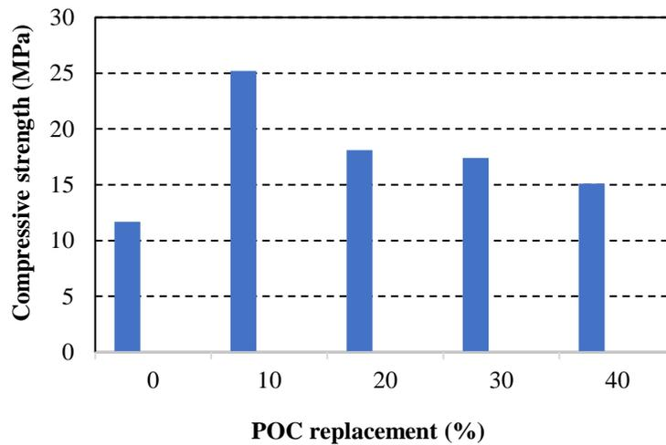
Figure 4. Compressive strength of mortar containing various percentages of POC
