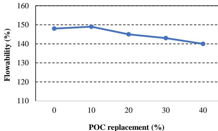
Figure 3. Flowability of mortar containing various percentages of POC
