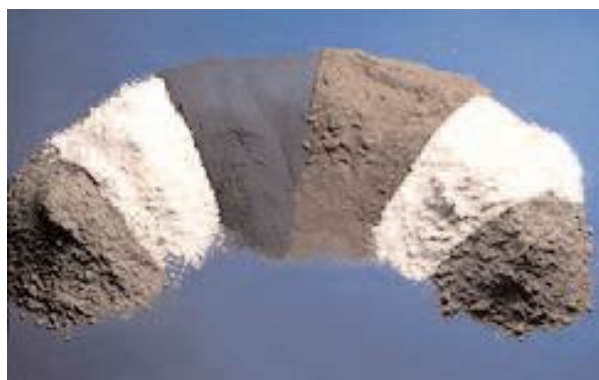
Figure 1. Type of cementitious materials: From left to right, fly ash (Class C), metakaolin (calcined clay), silica fume, fly ash (Class F), slag, and calcined shale [1]
