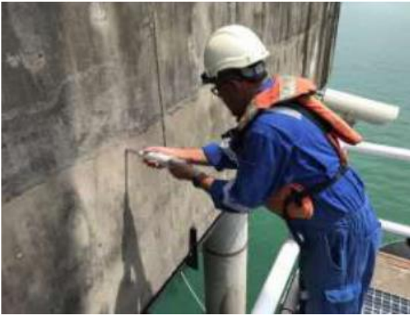
Figure 4. Rebound hammer test for concrete structure at loading platform
