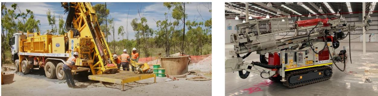
Figure 3. Advanced drill rig technology – truck mounted with automatic SPT hammer [16][19]
