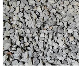
Figure 4. Natural coarse aggregate
