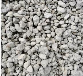
Figure 3. Recycled coarse aggregate
