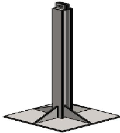
Figure 7. Load transfer column attached with base plate
