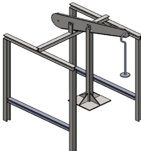
Figure 10. CAD model of field plate load test device
