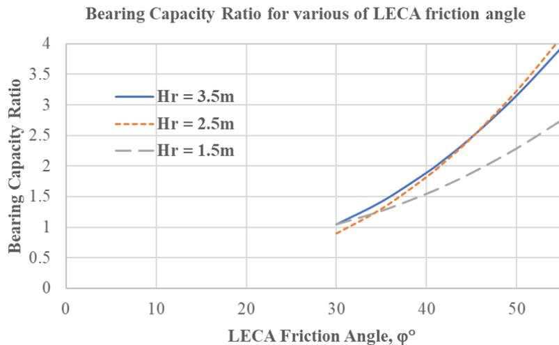
Figure 6. Bearing capacity prediction chart for various LECA replacement depth
