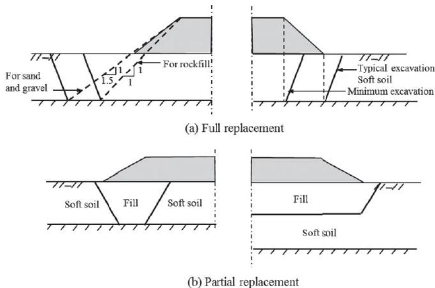
Figure 1. (a) Full and (b) Partial replacement under an embankment [4]
