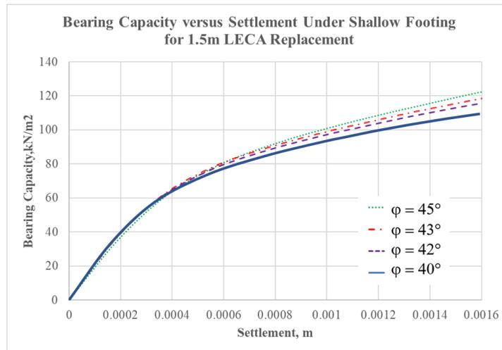
Figure 2. Bearing capacity of soft soil reinforced with 1.5m LECA raft
