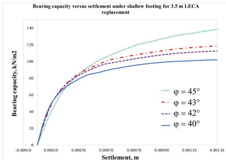
Figure 4. Bearing capacity of soft soil reinforced with 3.5m LECA raft
