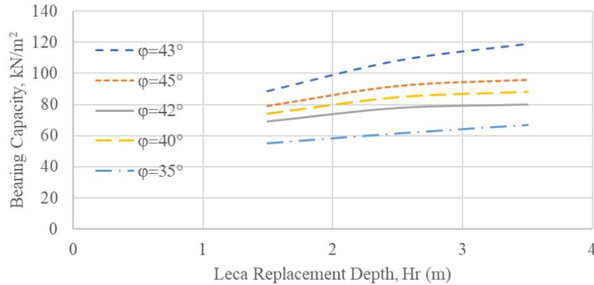
Figure 5. Bearing capacity for various LECA replacement depth
