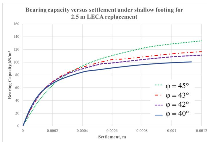
Figure 3. Bearing capacity of soft soil reinforced with 2.5m LECA raft
