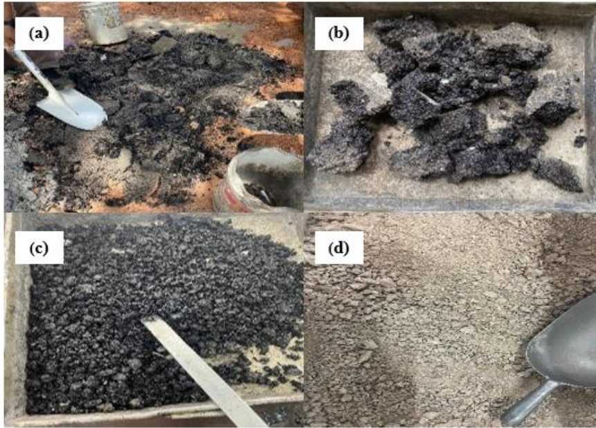
Figure 2. Process of extracting the aggregate from RAP samples
