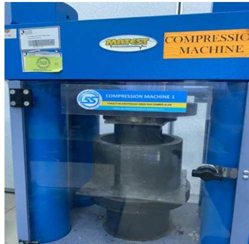
Figure 4. ACV compression equipment
