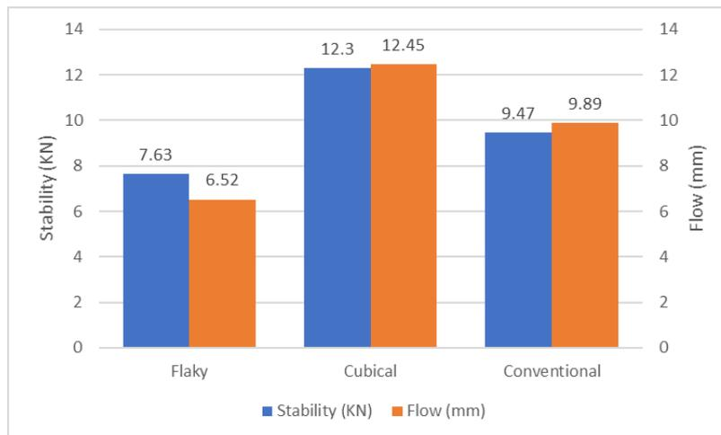
Figure 1. Result of Marshall Stability test
