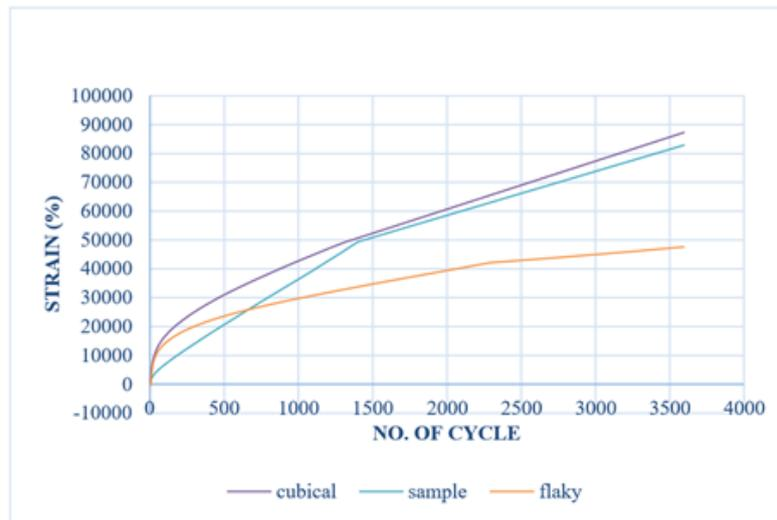
Figure 3. Result of Dynamic Creep test at 45°C
