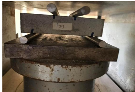
Figure 13. Prism specimen prepared to be tested.
