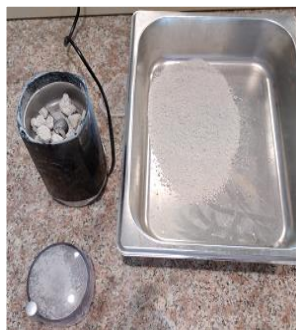
(b) Crushing lightweight pumice coarse aggregate to fine aggregate
