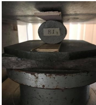
Figure 11. Specimen prepared to split tensile test.
