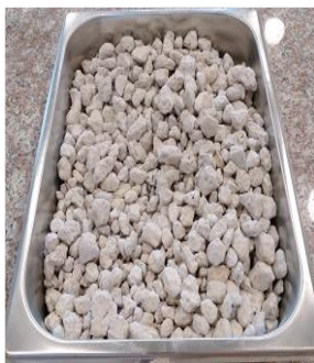
(a) Lightweight pumice coarse aggregate
