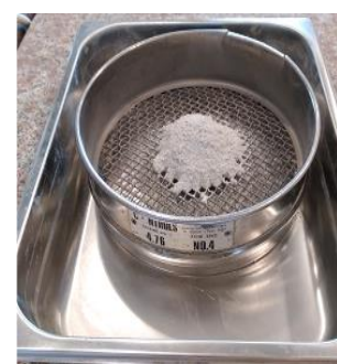
(c) Sieving lightweight pumice fine aggregate
