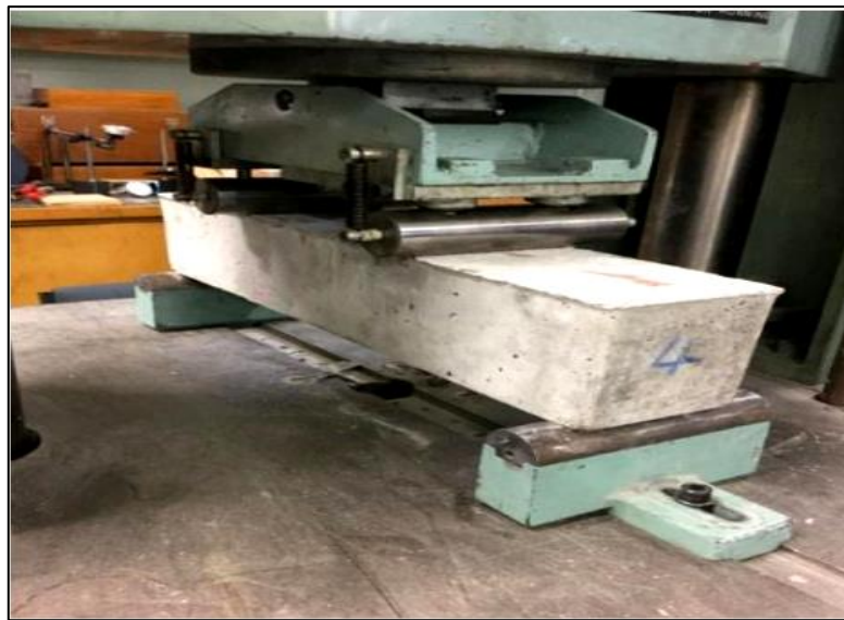
Figure 2. Test setup using Universal Testing Machine [17].
