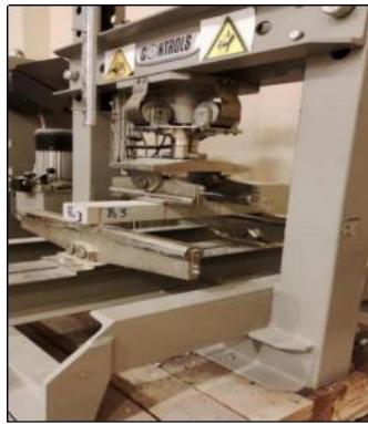
Figure 2: Loading set-up composite plain concrete beam
