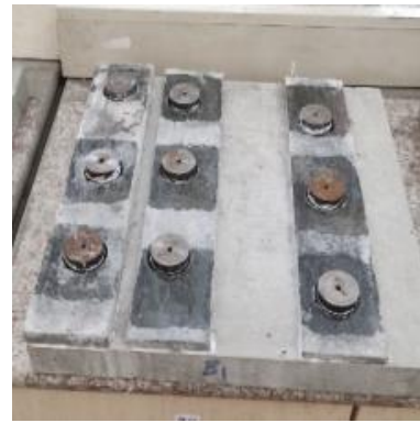
(b) cores execution and attached instrument dolly
