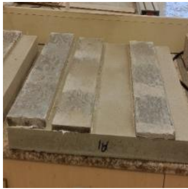
(a) Attached NSC substrate with UHPFRC strips
