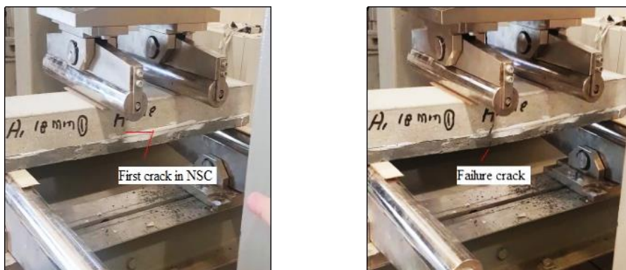
Figure 3: First crack start and failure crack width development of composite plain beam under flexural test
