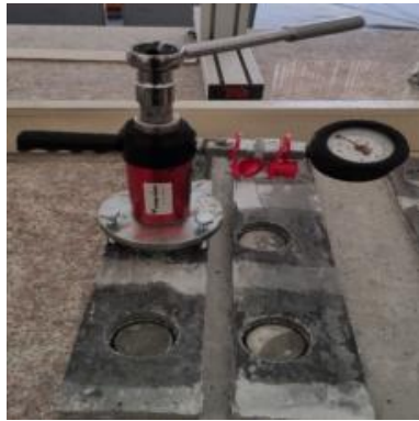
(c) pull-off by applying direct tension force on the dolly
