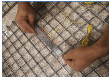
Figure 16. Location of strain gauges on reinforcement of slab specimens.
