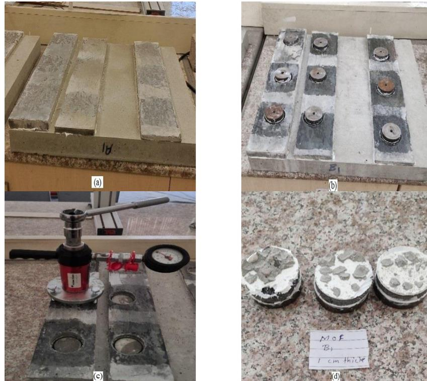
Figure 3. Pull-off test phases.
