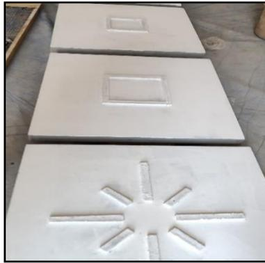
**Figure 4.** Strengthened NSC slab specimens by different distribution patterns of UHPFRC strips.
