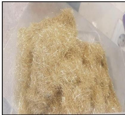
**Figure 2.** Straight copper-coated micro steel fibers.
