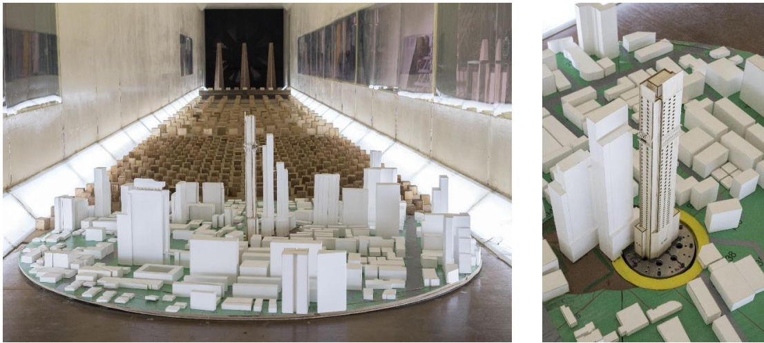
Figure 13. Overall wind load study of Park Thonglor in Bangkok, Thailand, by wind tunnel test and high-frequency force balance model.
