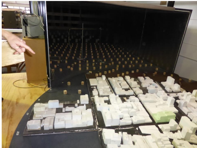
Figure 4. WSP \frac{3}{4} open-jet boundary layer wind tunnel at Petone, Wellington, New Zealand.
