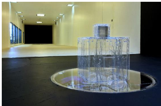
Figure 13. Windcatcher building model in the University of Auckland BLWT wind tunnel.
