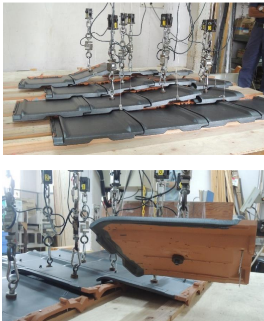
Figure 11. Pulling-up load test of clay tiled roof.
