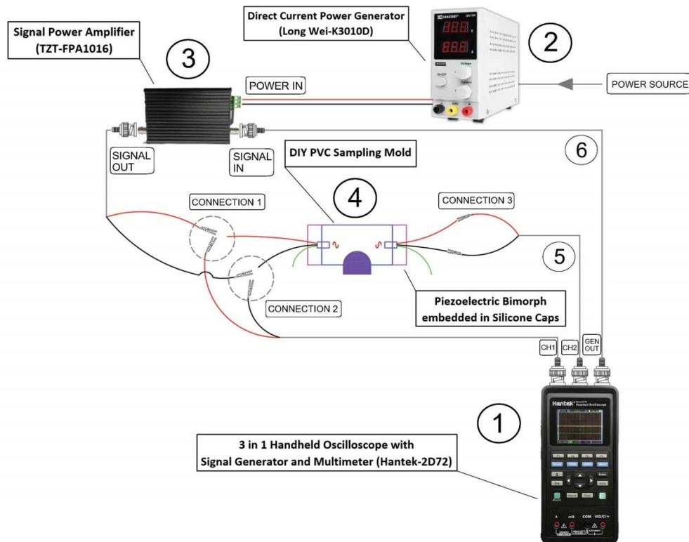
**Figure 2.** Schematic diagram of components proposed instrumentation setup.
