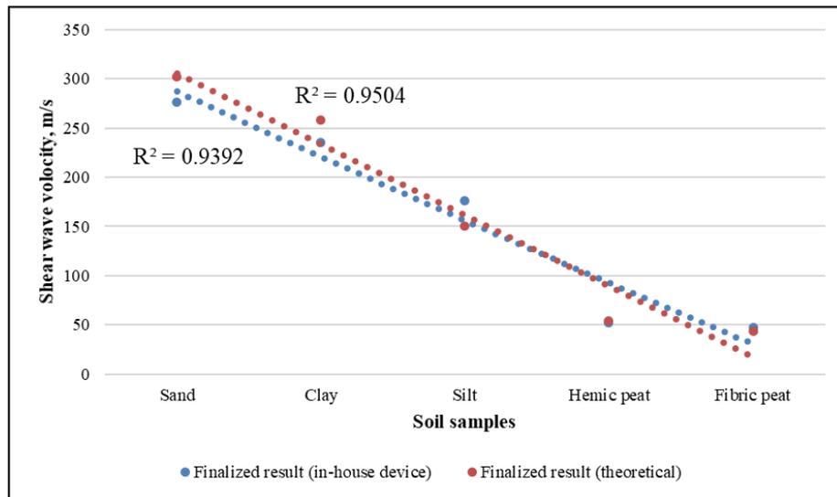
**Figure 3.** Theoretical and experimental data on various samples (best fit).
