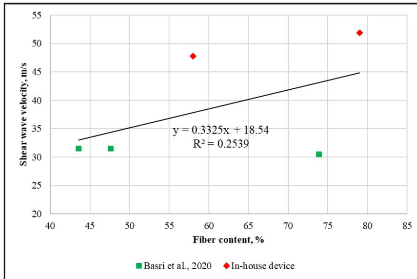
Figure 7. Shear wave velocity versus fiber content of peat.
