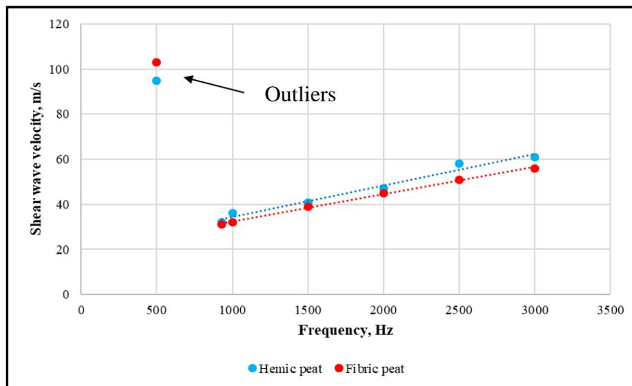
**Figure 4.** Shear wave velocity versus frequency on hemic and fibric peat sample.
