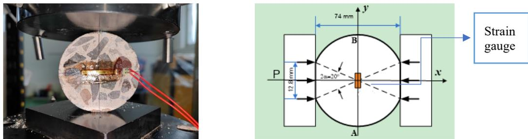
Figure 2. Schematic diagram of concrete split-tension loading method
