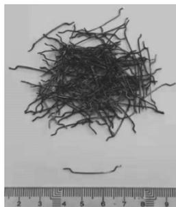
Figure 1. End-hooked steel fiber
