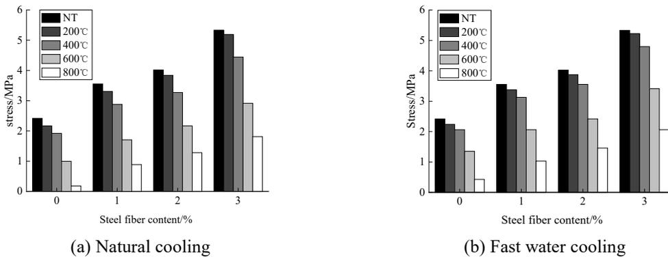
Figure 7. Effect of different temperatures on splitting strength of steel fiber concrete
