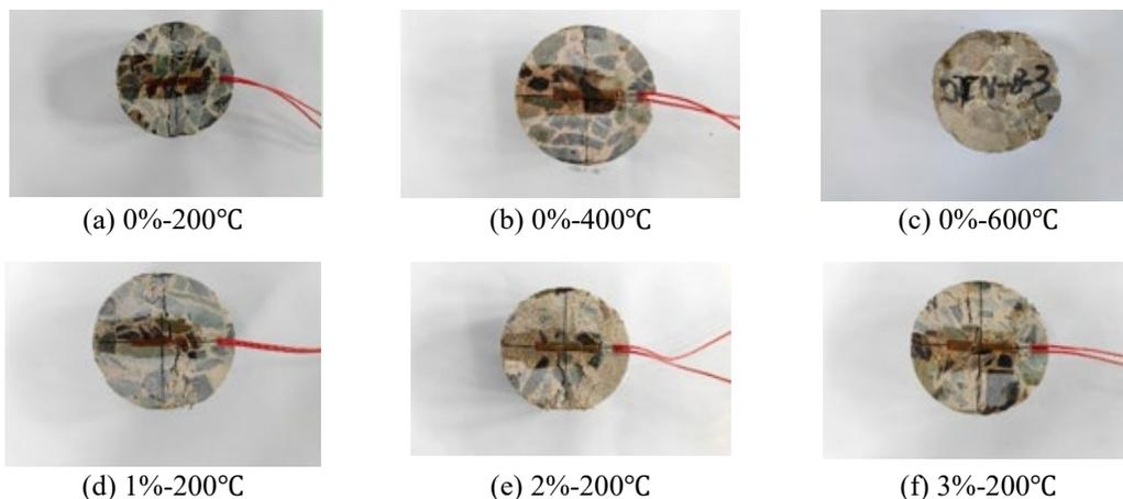
Figure 3. Split-tension damage pattern of steel fiber concrete under natural cooling mode
