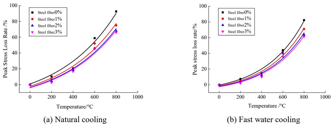
Figure 5. Effect of temperature on the rate of loss of peak stress in split tensile steel fiber concrete
