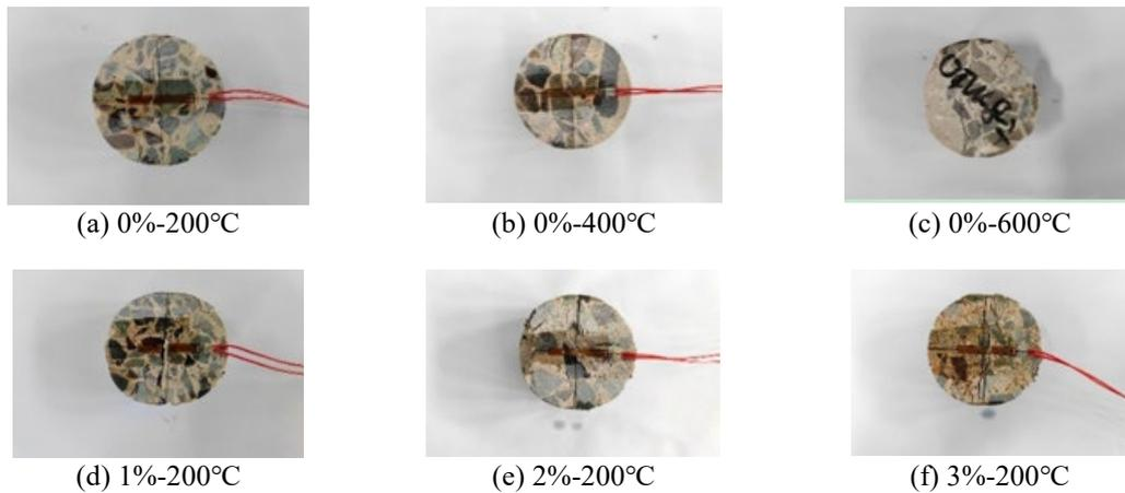
Figure 4. Split-tension damage pattern of steel fiber concrete under rapid water-cooling mode
