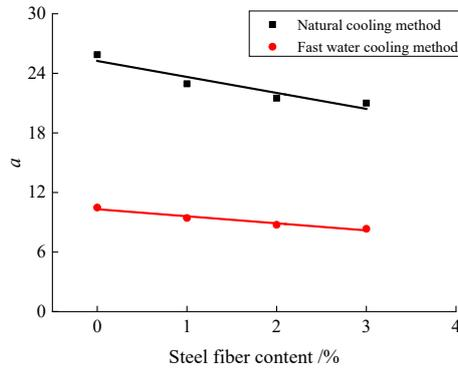
Figure 6. Relationship between steel fiber dosage and parameter a
