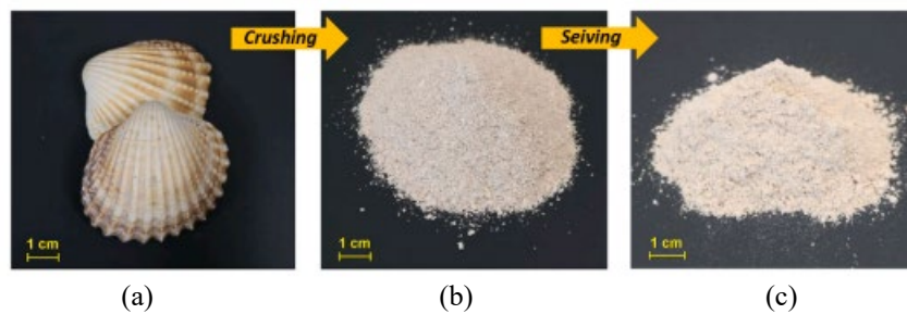
Figure 1. Preparation of seashell waste powder [32]
