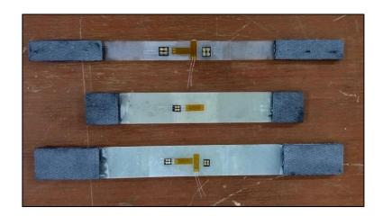
Figure 1. Specimens with tabs (in black) and strain gauges installed (from top to bottom: tensile  $0^{\circ}$ , tensile  $90^{\circ}$  and shear).
