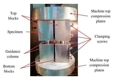
Figure 2. Compression jig setup with the specimen in between.
