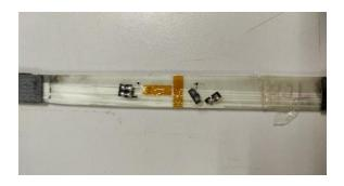
Figure 4. Failure mode of T-0 specimen.
