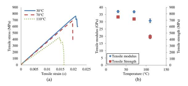
Figure 3. (a) Representative stress vs. strain curve comparison at different temperatures and (b) tensile modulus and tensile strength (with standard deviation) vs. temperature for T-0 specimens.
