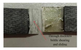
Figure 10. Failure mode of C-90 specimen.
