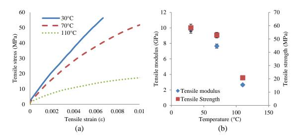
Figure 5. (a) Representative stress vs. strain curve comparison at different temperatures and (b) tensile modulus and tensile strength (with standard deviation) vs. temperature for T-90 specimens.
